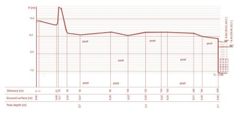
Figure 156. Surface character in west-east direction, before surface levelling. Sketch by J. Nusbaums.
