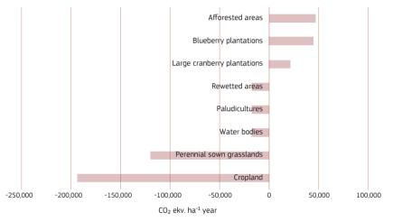
Figure 179. GHG emission reduction potential (CO<sub>2</sub> equivalents) of various after-use scenarios (10 hectares, 10-year period).
