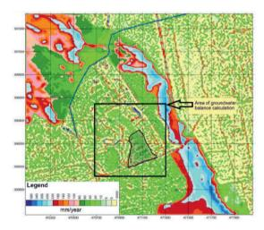
Figure 75. Map of water supplementation resulting from vertical filtration (mm/year) in the modelled unconfined aquifer (Q2) in Ķemeri Mire study area. Author of map: 0. Aleksāns.
