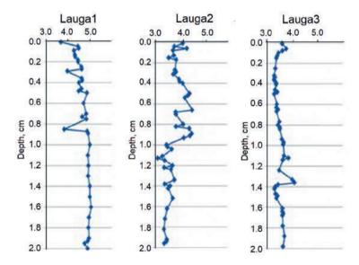
Figure 49. pH values in upper peat interval (0.0-2.0 m) of boreholes "Lauga1", "Lauga2" and "Lauga3".
