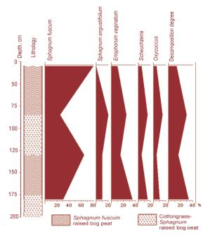
Figure 51. Botanical composition and peat decomposition degree in Drabiņu Mire, borehole "Drab1".
