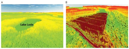
Figure 67. Examples of LiDAR three-dimensional data sets. A – part of Lauga Mire; B – part of Ķemeri Mire. Author of maps: O. Aleksāns.
