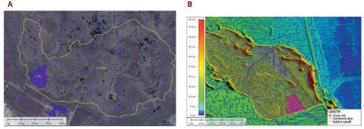
Figure 70. Catchment areas in the study areas, determined with three-dimensional model: A – catchment area of Lake Višezers in Lauga Mire; B – catchment area in part of Ķemeri Mire. Author of maps: O. Aleksāns.
