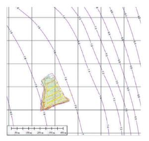
Figure 74. Modelled groundwater tables in aquifer Q2 (metres above the sea level) in Ķemeri Mire modelling area. Author of map: O. Aleksāns.
