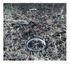
Figure 140. Greenhouse gas measurement site in tree plantation. Photo: S. Neimane.
