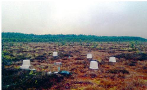
Figure 15. Opaque flux measurement chambers. Photo: I. Bebre.
