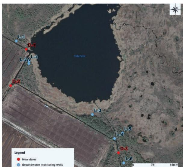
Figure 172. Locations of planned dams and piezometers installed within LIFE REstore project in Lauga Mire around Višezers Lake. Map prepared by A. Rudusāne. Orthophotomap at scale 1:10,000, 2013–2015, © Latvian Geospatial Information Agency.
