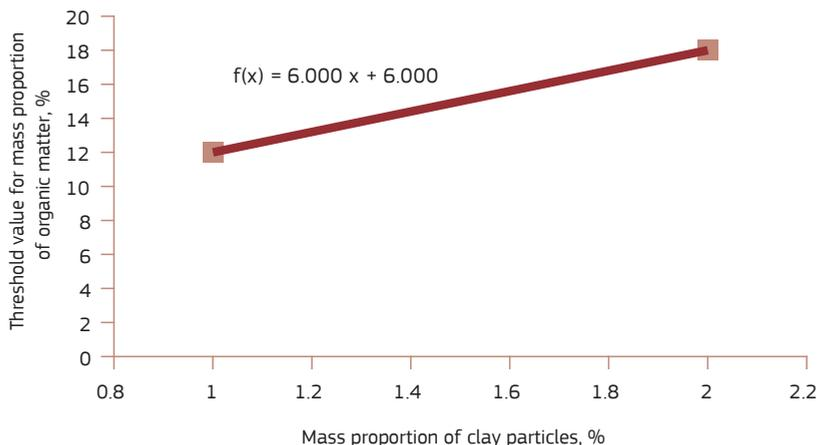
Figure 1. The limiting value of organic carbon in soils, which are periodically or permanently saturated with water, depending on clay particle content in soil parent material (Eggleston et al. (eds.) 2006).
