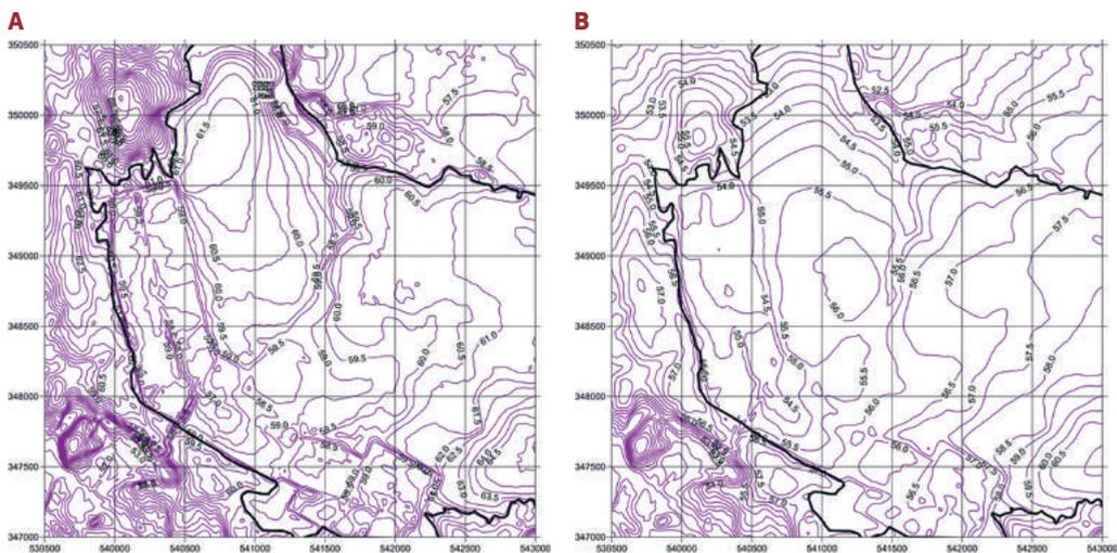
Figure 69. Modelled water tables at mire bottom B1 and in till gQ (Lauga Mire): A – groundwater table in Layer B1 (metres above the sea level); B – groundwater table in Layer gQ (metres above the sea level). Author of maps: O. Aleksāns.
