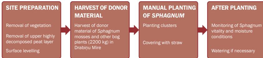
Figure 161. Works carried out in the demo site.
