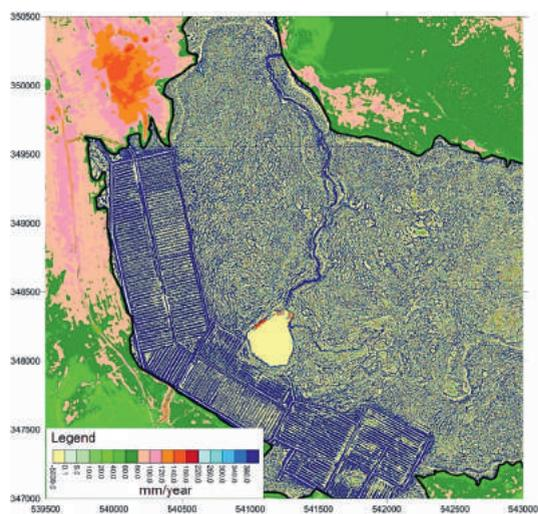
Figure 71. Supplementation of simulated mire sediment Layer B3 with atmospheric precipitation in a result of vertical infiltration (mm/year). Author of map: O. Aleksāns.
