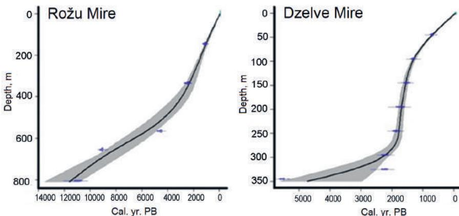
Figure 38. Curves of age-depth models characterizing the intensity of peat accumulation in raised bogs – Rožu and Dzelves Mires (Kalniņa et al. 2013).
