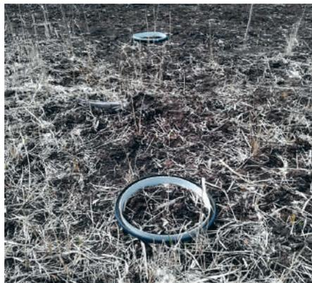
Figure 140. Greenhouse gas measurement site in tree plantation. Photo: S. Neimane.
