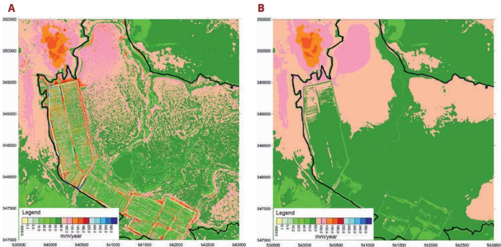
Figure 72. Supplementation of modelled water supply as a result of vertical filtration from upper layer (mm/year): A – peat sediment Layer B2; B – peat sediment Layer B1. Author of maps: O. Aleksāns.
