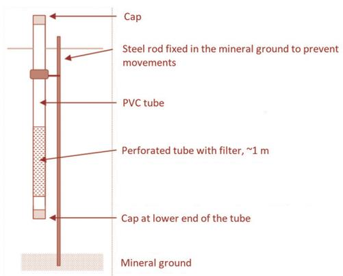
Figure 163. Construction of piezometer with a fixed rod to prevent movement. Drawing: Dēliņa (2014).
