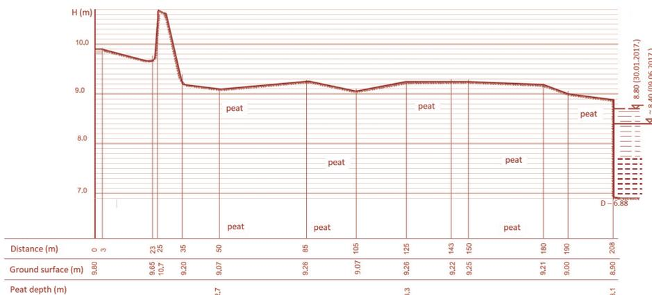
Figure 156. Surface character in west-east direction, before surface levelling. Sketch by J. Nusbaums.
