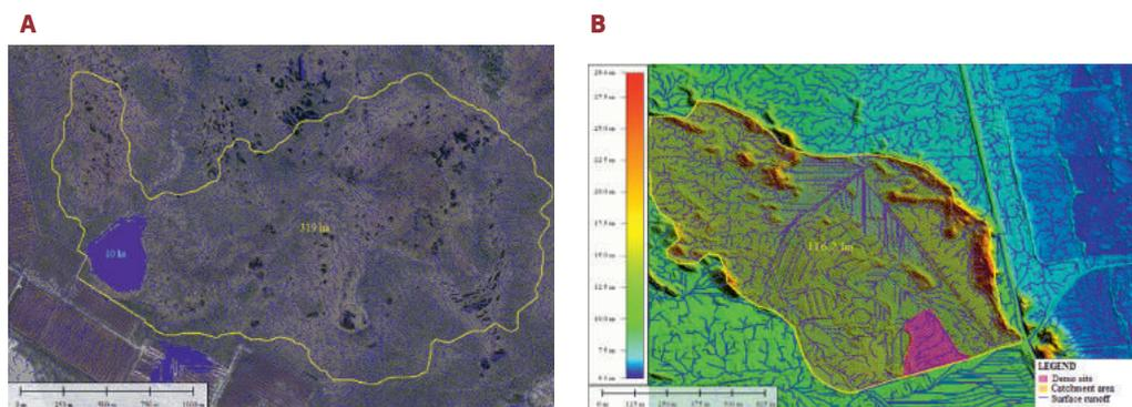
Figure 70. Catchment areas in the study areas, determined with three-dimensional model:
